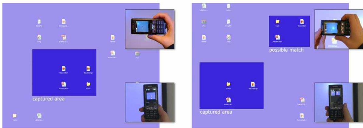
Figure 3. Left shows the prototype with one possible match. Right shows the interaction with two identical icon constellations on the desktop. The magnifications denote the capturing process (top) and the result shown to the user (bottom).
