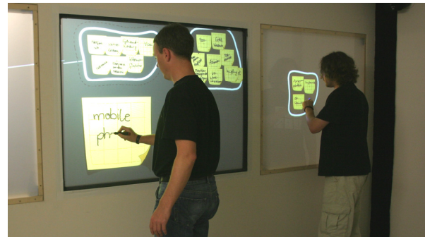
Figure 8. Our variable precision input system with one user doing fine-grained interaction and another using coarse tracking for organization.
