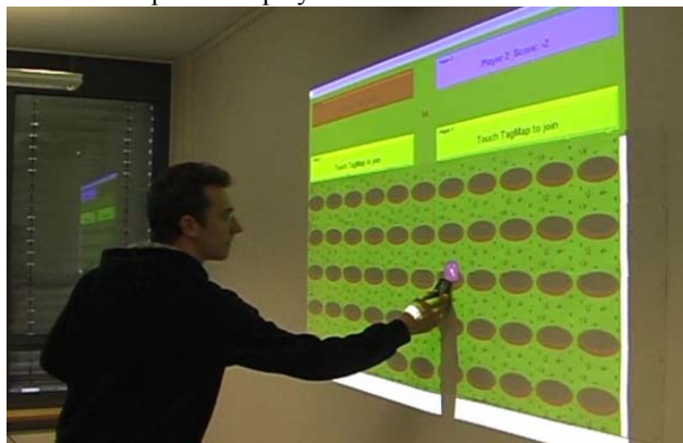
Fig. 1. Direct, touch-based interaction with a dynamic NFC-display
