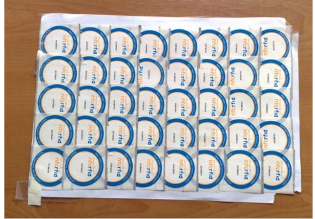
Fig. 3. Backside of a tile of the NFC-grid with 8 by 5 overlapping tags
