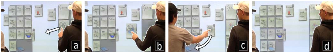
Figure 13. Drag between a public intermediary. (a) person drags note out of his personal interaction area, (b) using the empty space between the interaction areas as a clipboard. (c) second person drags note into his interaction space of the tablet, and (d) the note is now moved to his tablet.
