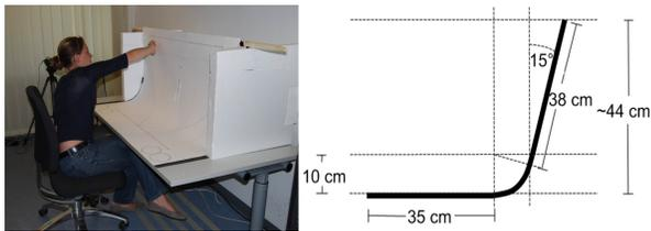
Figure 2. left: A study participant trying to reach the upper left corner of the prototype. right: Suggested measures of *Curve*.
