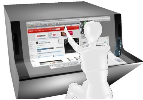
Figure 1. The Curve concept combines a horizontal and a vertical interactive surface, merging physical and virtual desktop.
