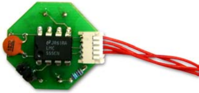
Figure 4. A sensor board, measuring only 20x20mm. It is connected to the CapBoard with a 4-wire cable. Different sensor electrodes can be attached to accommodate space limitations and range requirements.
