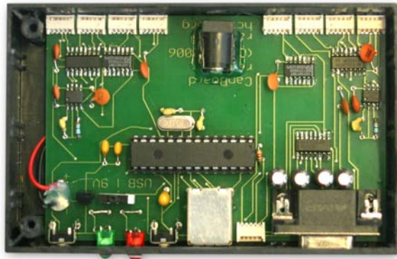
Figure 3. The CapBoard is assembled from standard parts. A PIC 18F2550 microcontroller controls the two sensor circuits and sends measurement data via USB. A connector for an external power supply and four freely programmable I/O pins enable stand-alone operation.
